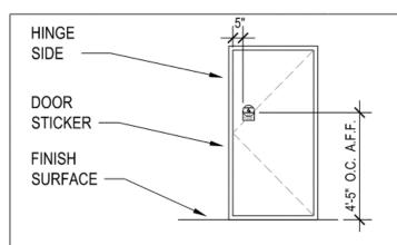
NOTE: STICKER SHALL BE PLACED ON EACH SIDE OF THE DOOR BEING OPENED, AT THE SPECIFIED HEIGHT. EXACT STICKER PLACEMENT LOCATION MIGHT BE DOOR SPECIFIC. CHECK WITH
